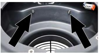
→ Unscrew the nuts of the rear fastener.
