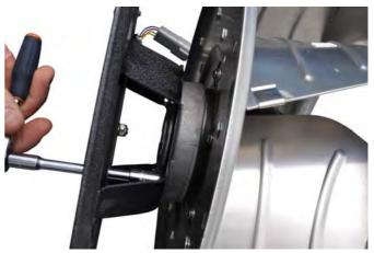
→ Unscrew the screws of the fan wheel/motor on the motor support.
