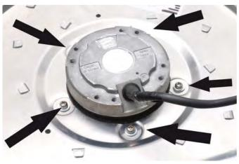
→ Unscrew the screws of the motor.
